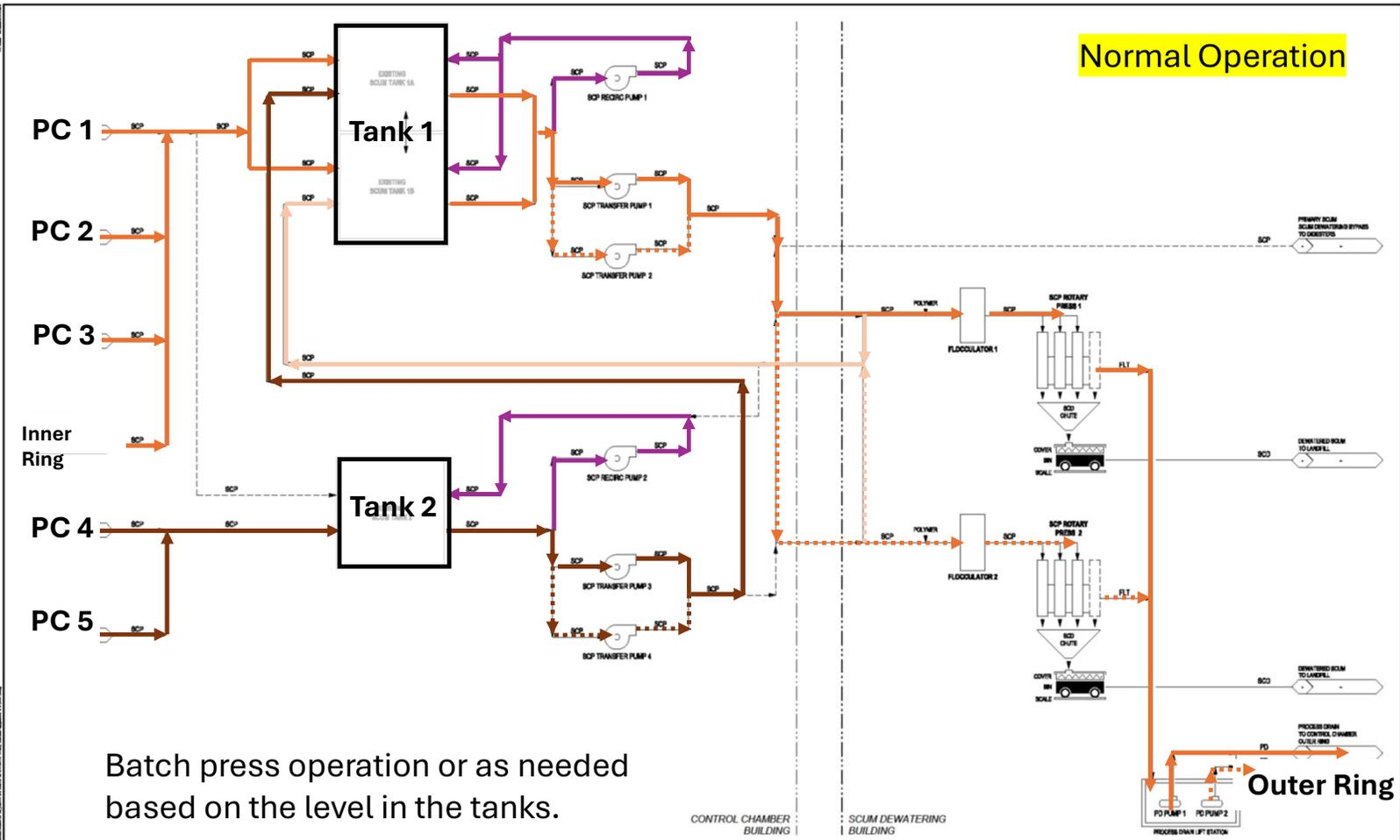
Batch press operation or as needed based on the level in the tanks.
